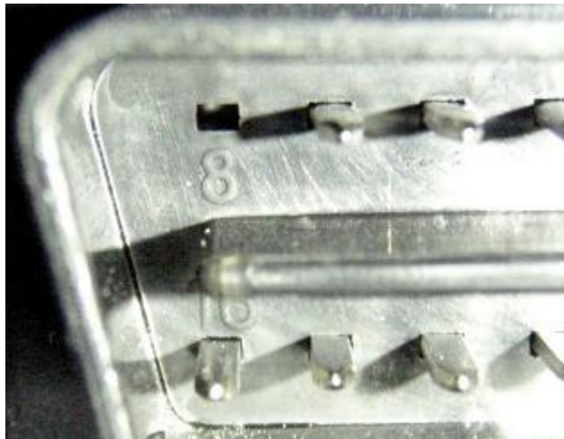
Close-up Picture of an Interface with pin8 removed (Second Generation)
